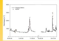
culated discharge by the ADiGS was within 20 percent compared to the gauging station. From the middle of May until beginning of June the discharge values were not reliable because of several technical problems. The measurements in June and July are very close to the observed discharge. During this time the activating of the system due to changing water levels was tested and demonstrates the potential of measuring many different discharges within a short time.
