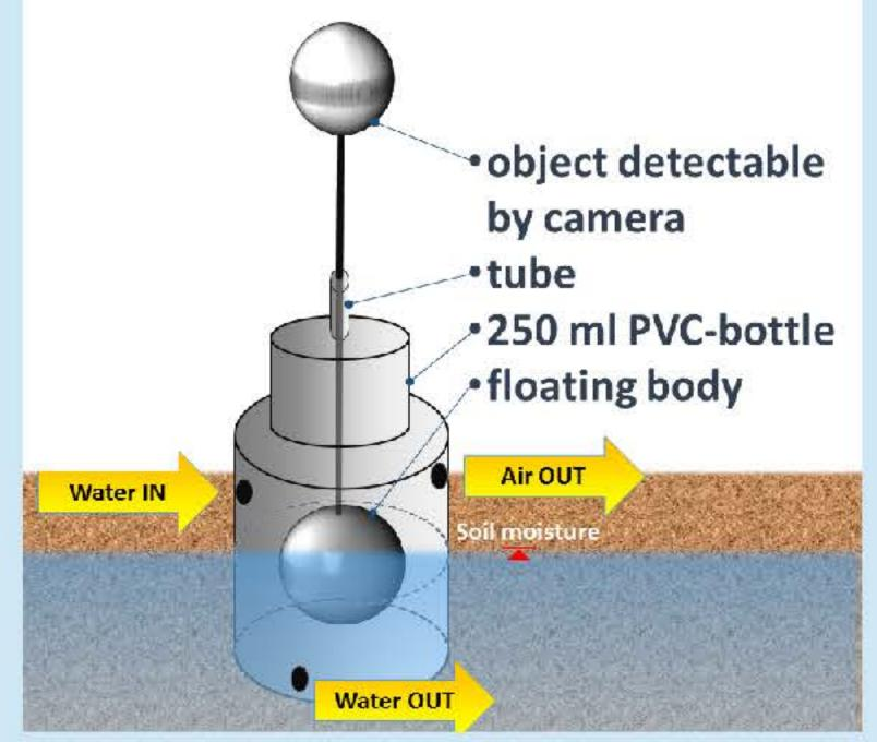
The soil saturation sensor consists of a 250 ml PVC bottle with holes for water in- and out-take. In the bottle a floating body will be risen during higher water level. That floating body is connected with a carbon fiber stick to a marker ball whose position can be monitored by the camera. A tube will ensure the upright posi-
