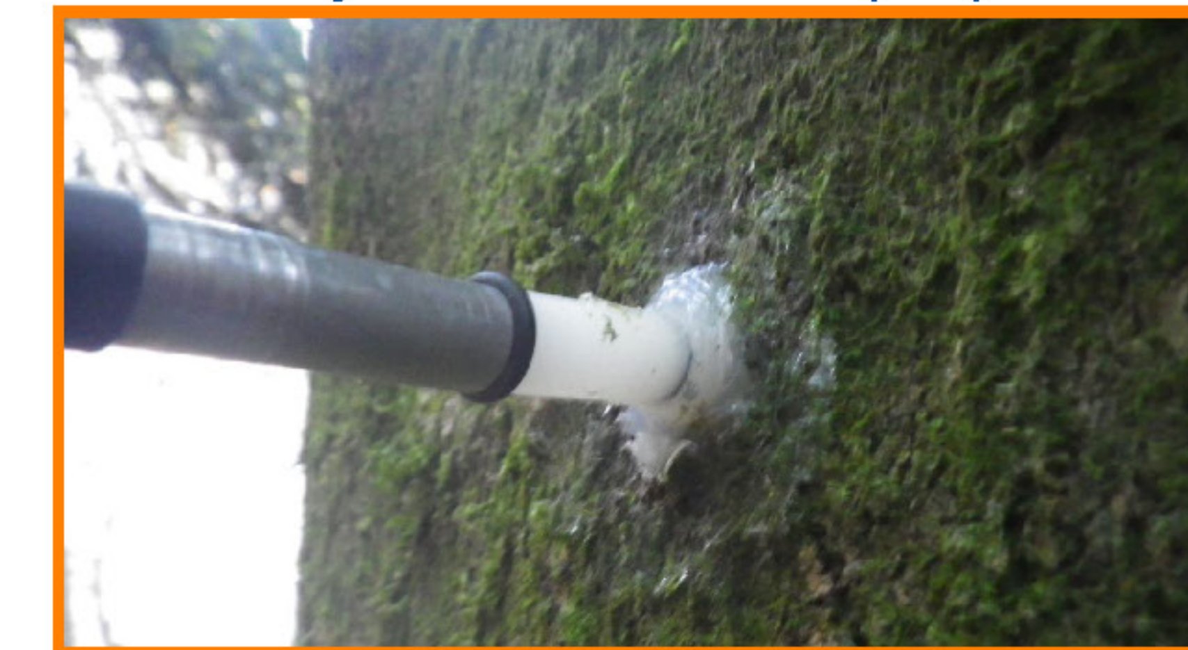
XWIP: Xylem water isotope probe
